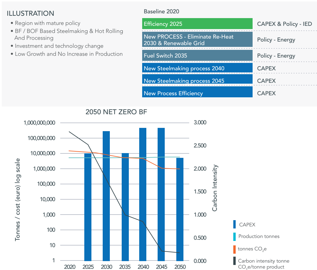
Figure 17: Illustration of a 2050 pathway for an integrated BF/BOF steel producer with technology deployment and CAPEX requirements
